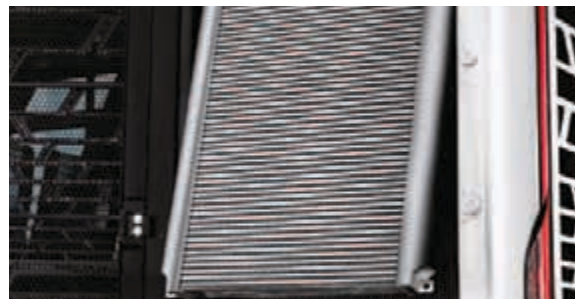
Easy cleaning of radiators thanks to the tilting intercooler.
