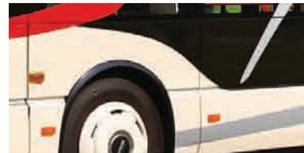
Each body panel is screwed for easy and fast replacement.
